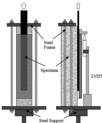
Fig. 3. Test setup for the direct shear test
