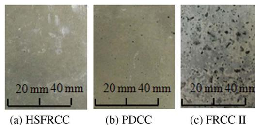
Fig. 4. Surface of FRCC plate
