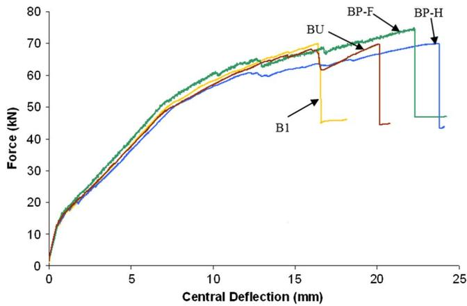
**Fig. 9.** Comparison of residual load after FRP debonding in the strengthened beam with unstrengthened beam (Lee et al. 2004, reprinted with permission from The Hong Kong University of Science and Technology)
