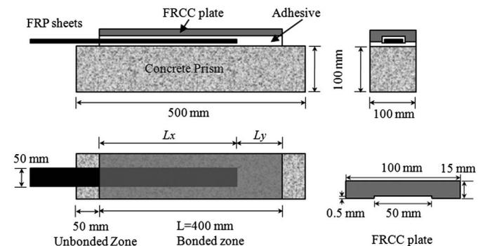
**Fig. 2.** Test specimen and FRCC plate with detailed dimensions
