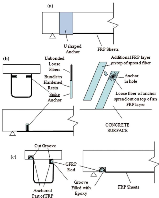
**Fig. 1.** Various approaches to anchor the FRP strip: (a) U-shaped anchor; (b) spike anchor; (c) NSM FRP anchor
