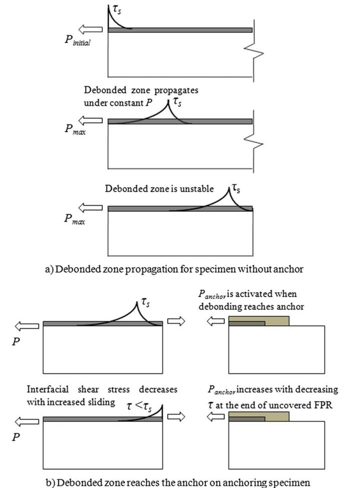
**Fig. 11.** Debonded zone propagation and shear softening
